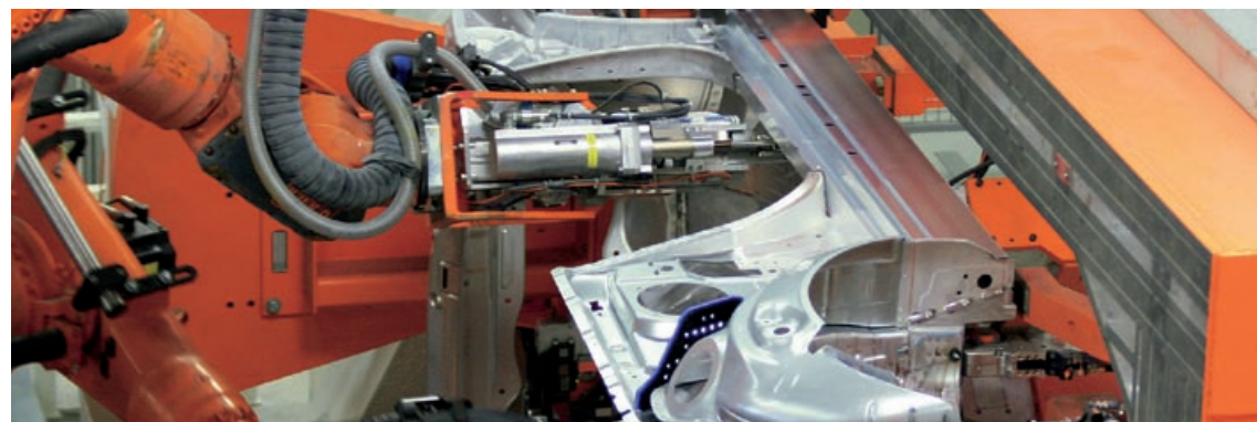
All in one cycle: Position the screw, create the hole, roll the thread, run the screw down and tighten up to a predefined torque.
