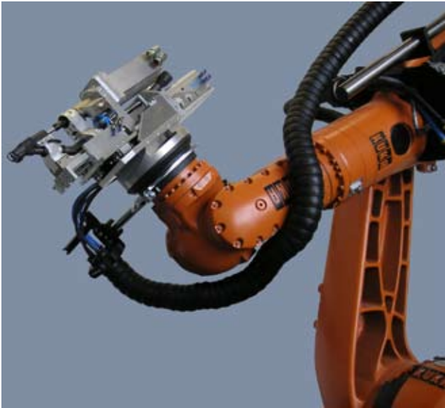
Robot-assisted fastening system supplied by Weber Schraubautomaten
