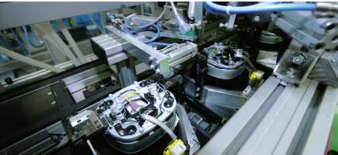
Assembly and test technology in one. In airbag assembly, the highest safety demands are made on material and processing.
